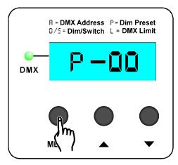
Once the **Dimmer Preset** settings are complete, press the **MENU** button to return to the **DMX Address Mode**.
