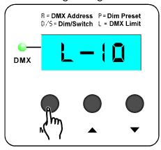
Press the **UP** or **DOWN** buttons to change the value within the range of **10% - 100%.** Each press of the **UP** or **DOWN** buttons will change the value by a single digit. Pressing and holding the **UP** or **DOWN** buttons will change the value quickly by multiple digits. Once a specific value has been selected, it will be saved automatically.
