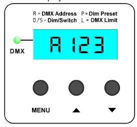
Each press of the **UP** or **DOWN** buttons will change the DMX address by a single digit. Pressing and holding the **UP** or **DOWN** buttons will change the DMX address quickly by multiple digits. Once a specific DMX address has been selected, it will be saved automatically. **NOTE: OUTPUT IS DISABLED DURING DMX ADDRESSING!**
