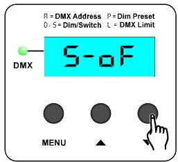
Once the **Dim/Switch Pack** settings are complete, press the **MENU** button to return to the **DMX Address Mode**.
