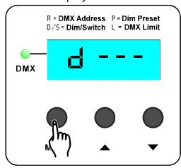
The Dim/Switch mode can be changed by pressing the **UP** or **DOWN** buttons. Doing so the LED display will show **S---** which means the **Switch Pack Mode** is activated.
