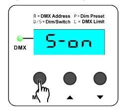
In the Switch Off Mode, output is turned off and the fixture is controlled by DMX signal. When DMX level is less than 40%, the fixture goes out; when DMX level exceeds 40%, the fixture lights. You can adjust the level by adjusting the Local Dim Knob.
