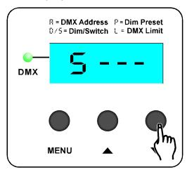
Press the **MENU** button to confirm the **Switch Pack Mode**, and then select **Switch On (S-on)** or **Switch Off (S-of)**. In **Switch On Mode**, the output is turned ON and fixtures light regardless of DMX signal.
