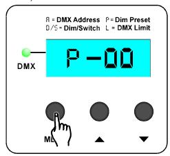
Press the **UP** or **DOWN** buttons to change the value within the range of **00% - 100%**. Each press of the **UP** or **DOWN** buttons will change the value by a single digit. Pressing and holding the **UP** or **DOWN** buttons will change the value quickly by multiple digits. Once the **Dimmer Preset** has been selected, it will be saved automatically.
